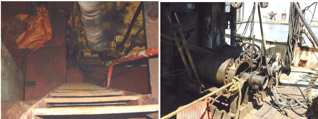
Figure 2.1. On-board hazards associated with commercial shrimp fishing as illustrated by steep and unsteady ladder descent in engine room compartments and on-deck unguarded machinery/winchs as well as low height of the deck railing. Reprinted with permission from J Agromedicine. 27
