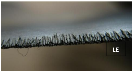
Figure 17. Compressor blade exposed to WDE process.
