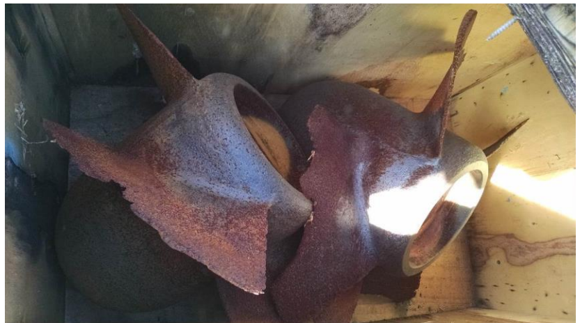
Figure 23. Pump C, used pump impellers (4000 hours of service). In both cases, large amounts of material were removed from the impeller due to the cavitation measured by the authors
