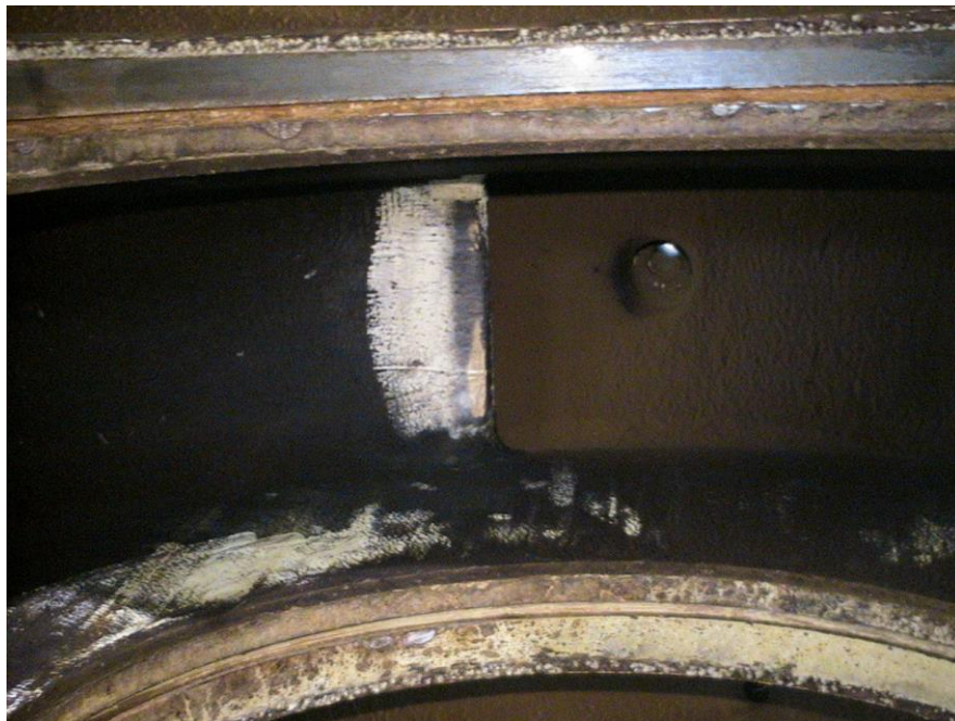
Figure 30. Pump F also exhibited cavitation damage on the wear ring exit (above), and the volute tongue (below). Accelerometer measurements on the casing indicated local acceleration peaks in these areas. The tongue erosion likely occurred due to discharge recirculation, since this pump often ran at 60% BEP flow.
