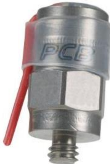
Figure 11. PCB Piezotronics Model M353B17 High Frequency, Quartz Shear ICP Accelerometer +/- 500 G's range, 30 kHz to 3 dB roll-off point, useful (but distorted) output to 100 kHz
