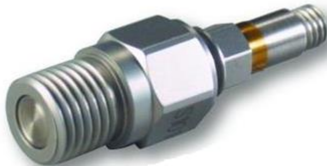
Figure 10. PCB Piezotronics Model 111A26 General Purpose ICP Pressure Transducer +/- 500 psi range, 400 kHz frequency response
