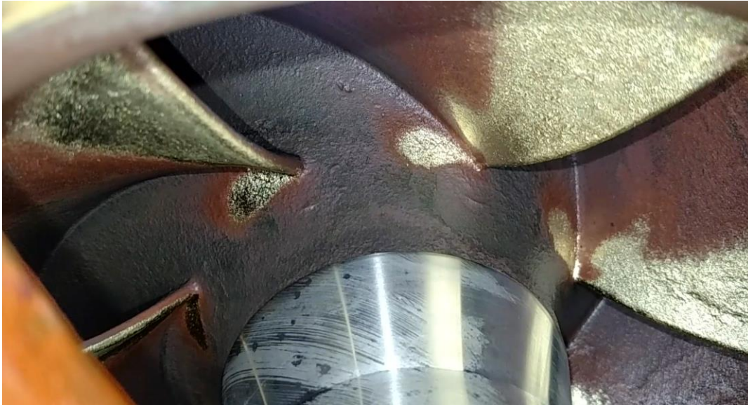
Figure 14. Pump A impeller picture. Note the polished surface of the low pressure side of the vanes which extends onto the hub.
