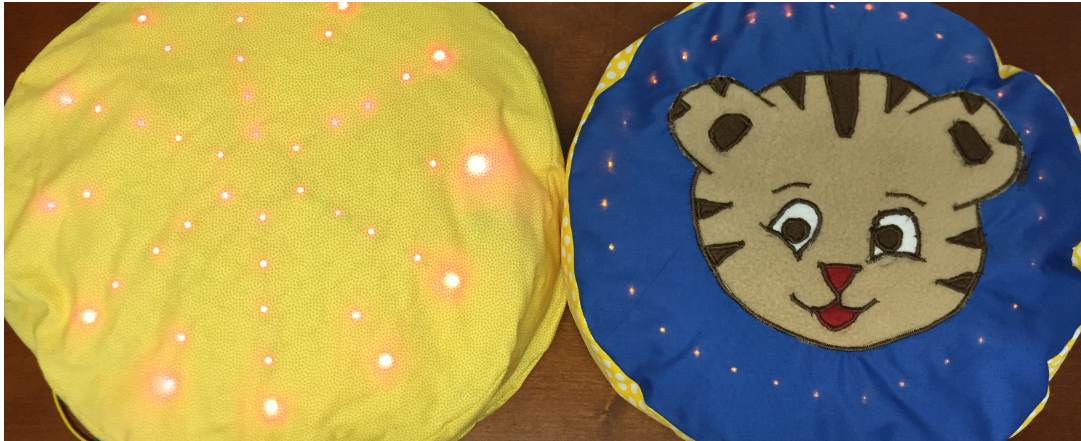
Figure 1: The above image shows the second iteration of the pillow prototype designs. They both have light feedback and use various wireless remotes to trigger the light patterns.
