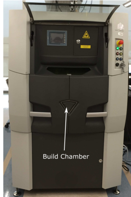
Figure 3.1: 3D Systems ProX 100 DMP L-PBF system. Reprinted with permission from [42].
