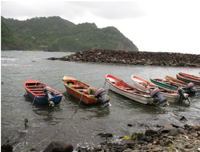
Figure 6. Boats moored at Desa Ikan during the data collection periods. This photo from 2015 shows the three types of boats moored at Desa Ikan, behind the stone wave breaker. The blue/orange boat on the far left is a wood keel boat, the orange boat that is second from the left is fiberglass with a wooden frame, and the white/orange boat that is third from the left is a fiberglass boat.
