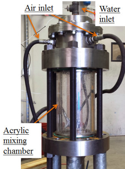
Figure 11. Gas-oil mixer with an acrylic mixing chamber
