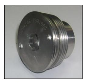
Balancing weight used for trim balance (off-the-shelf windage plug to be installed on flange stud bolts)
