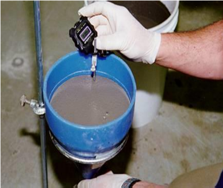
Figure 6: Measure the Time it takes for Grout to pass through the Flow Cone
