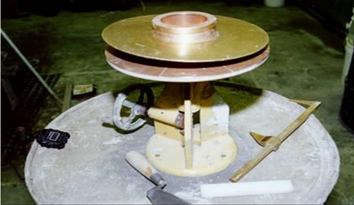
Figure 2: Precision Grout is placed into 4" (102 mm) ring mold and dropped 5 times within 3 seconds
