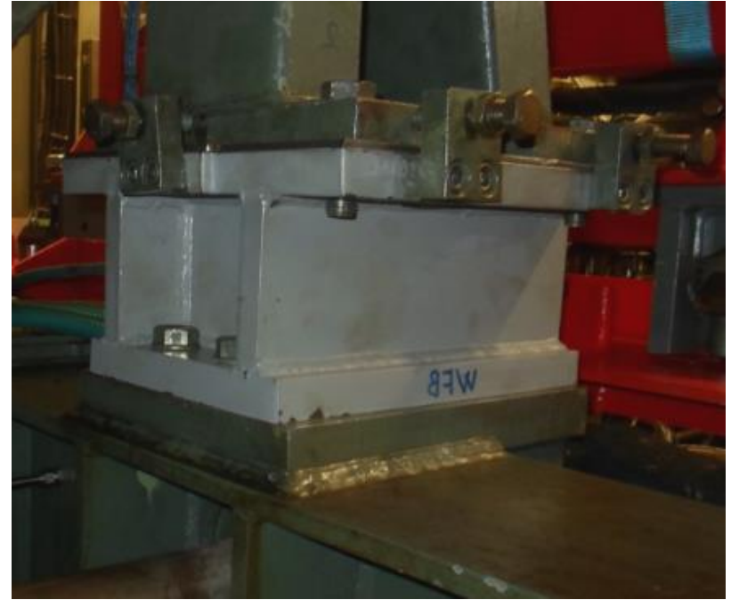
PT support after modification
