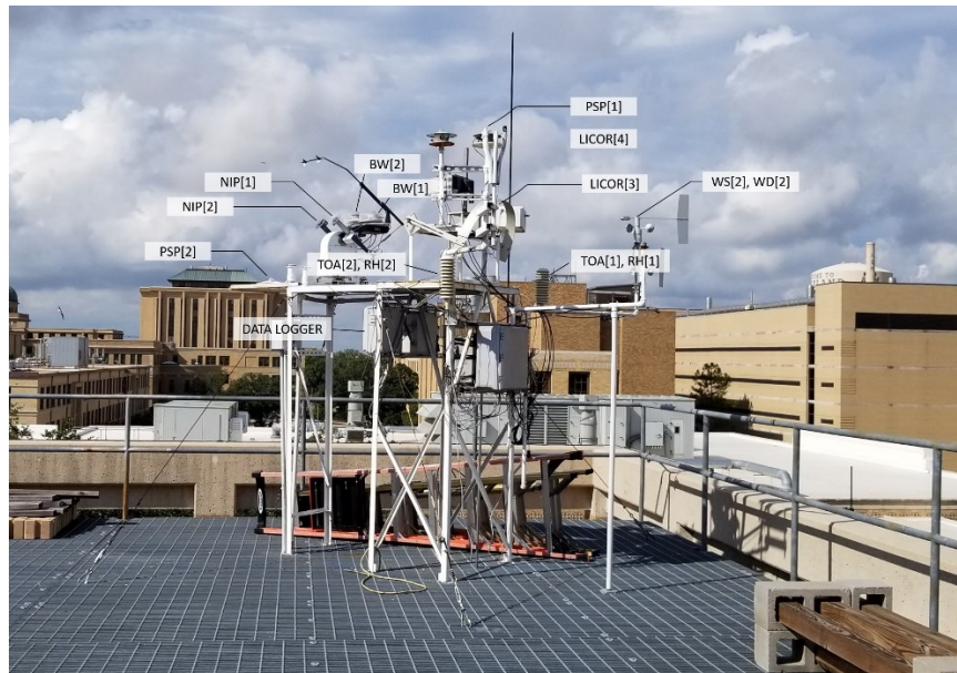
Figure 44. Exterior View of the Solar Test Bench
