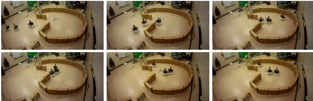
(a) Group of robots following the BOIDS motion model being corralled by static environment.
