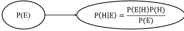
Fig 2.4 BN on causal relationship between the evidence (E) and the hypothesis (H) depicting the Bayes Theorem. Modified from Korb and Nicholson (2004). There might be multiple parents/children.
