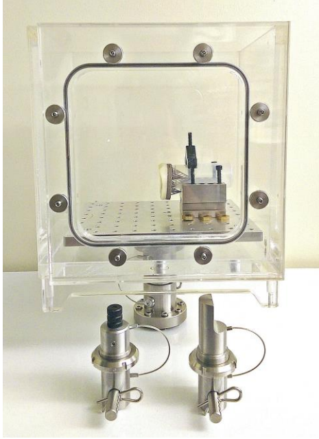
Figure 8: Interlock shear test setup in the A-P orientation (back), laser alignment device (front left), and indenter (front right). Consult Appendices 2,3,4,5,6,7,9 and 11 for further technical schematics of all fixtures.
