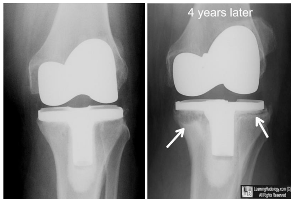
Figure 2: A radiographic image depicting the development of aseptic loosening in a current stemmed TKA. The white arrows indicate areas of decrease bone density, which result from stress shielding. Published with permission from LearningRadiology.com
