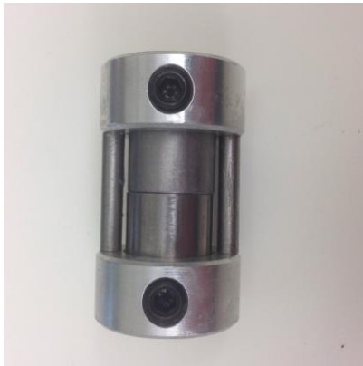
Figure 6: Shear fatigue sample in bonding jig during adhesion
