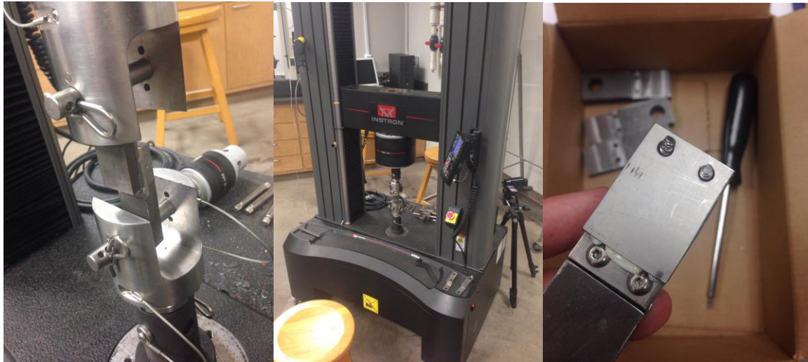
Figure 9. The left two photos are the setup using the Instron and the lap shear loading grips. The right-most picture is of the bolt failure that occurred as result of the testing.
