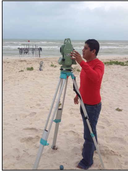
Figure 5. A team member taking beach profile elevation measurement during the field experiment.
