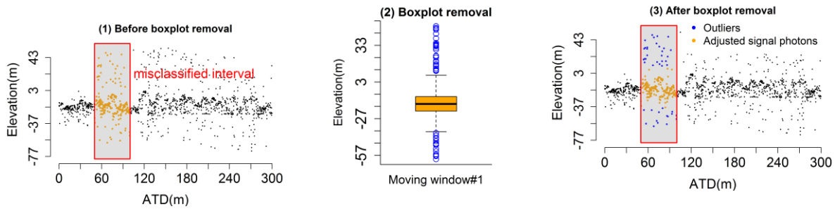
Figure V-8. An example of box plot removal filter for adjusting possible signal photons.
