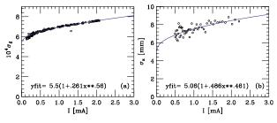
FIG. 5. (Color) Measurements of steady-state energy spread (a) and bunch length (b), with  $V_c = 300$  kV.
