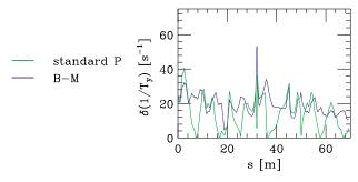
FIG. 1. (Color) Vertical steady-state (local) growth rate over 1/2 the ATF for an example with vertical dispersion due to random errors. Given are results due to standard Piwinski (green curve) and Bjorken-Mtingwa (blue curve).
