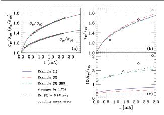
FIG. 6. (Color) ATF measurement data (symbols) and IBS theory fits (the curves). The symbols in (a) give the smooth curve fits to the measured data of Fig. 5.
