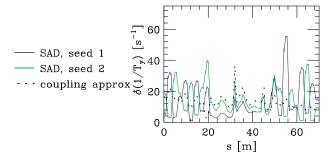
FIG. 3. (Color) Vertical steady-state (local) growth rate over 1/2 the ATF for an example with vertical dispersion and x-y coupling due to random errors. Given are results obtained by SAD (for 2 seeds; solid curves) and by the coupling approximation used here (dots).
