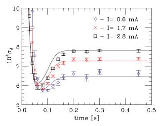
FIG. 4. (Color) Measured energy spread as function of time after injection, for three different currents (the plotting symbols). The curves give BM simulations assuming an *x-y* coupling of 0.006 and no potential well distortion. This plot is reproduced from Ref. [4].
