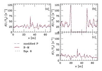
FIG. 2. (Color) Steady-state (local) growth rates over 1/2 the ATF for an example with vertical dispersion due to random errors. Given are results due to modified Piwinski, Bjorken-Mtingwa, and Eqs. (6).
