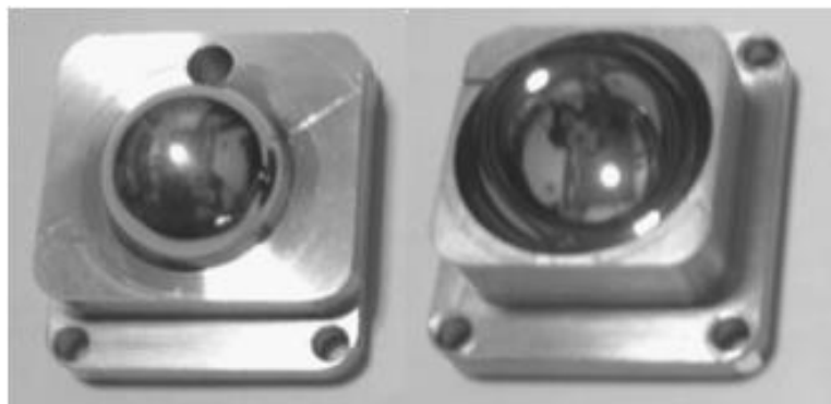
Figure 2.14: Plastic lens mould insert [57]
