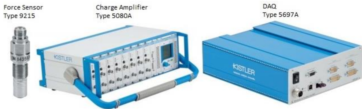
Figure 6.2: Kistler force measurement equipment
