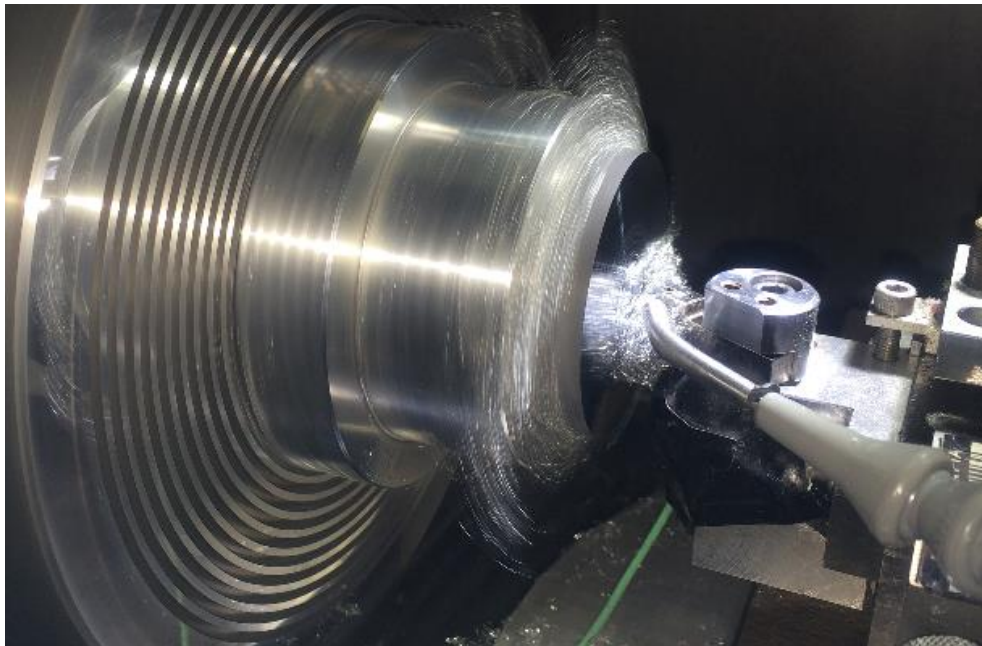
Figure 4.8: Chips around tool during low cutting speeds
