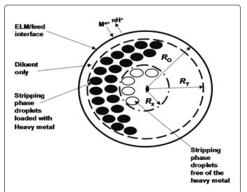
**Figure 2:** Schematic representation of an ELM globule in the shrinking-core model.  $R_{\rm O}$  is the overall ELM globule radius (m),  $R_{\rm Y}$  is the inner core radius of the ELM globule (m), and  $R_{\rm X}$  is the reactive front radius for a given ELM globule (m)
