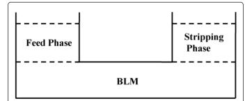
Figure 1: Schematic representation of the BLM system for metal extraction
