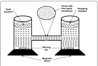
**Figure 4:** Schematic representation of an extraction apparatus containing a flat-sheet SLM.
