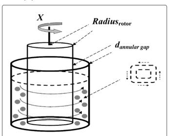
**Figure 3:** Schematic representation of the Taylor-vortex column. Symbols in the figure have identical meaning to those in equation 3 (see below). The ELM globules () become dispersed in the treated wastewater, i.e. the feed phase, through the rotation of the inner cylinder located inside the Taylor-vortex column. The figure was adapted from Park [50].
