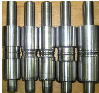
Fig. 4. Thorns on rolling bearing rings
