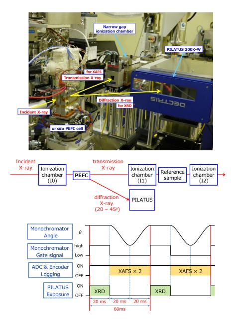
**Figure 1.** Experimental setup for *in situ* time-resolved XAFS and XRD measurements of PEFC Pt/C cathode catalysts under voltage operating conditions, a schematic diagram of the setup, a high-speed regulation pattern of monochromator angles with gate signals, and recording time charts of detectors for the simultaneous XAFS and XRD measurements
