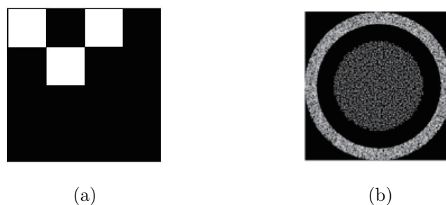
Fig. 4. (a) 9:16 symbol modulation code pattern. (b) Input digital data page with coded signal and reference patterns.
