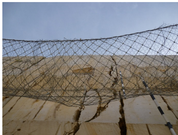
Figure 6. Displacement of the net towards the impact point evidencing some curtain effect.
