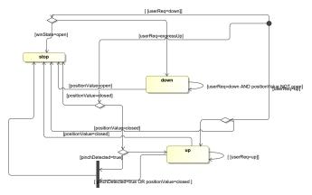
(c) SysML: State machine diagram that describes the behavior of the WinController IBD.
