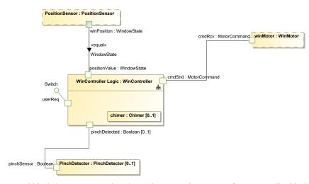
**(b)** SysML: Internal block diagram (IBD) that shows the internal structure of WinController block defined in the BDD.
