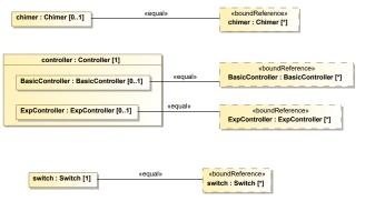
**(b)** SysML: Mapping of each component with variability (Chimer, BasicController, ExpController) to dedicated bound references.
