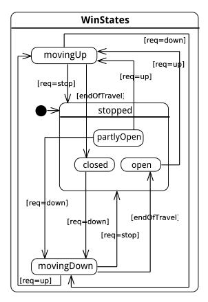
■ **Figure 4** UML state diagram for a control automaton for the power window controller.
