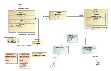
(a) SysML: Complete block definition diagram (BDD) of the power window subsystem showing all the relevant blocks, references, and value types.
