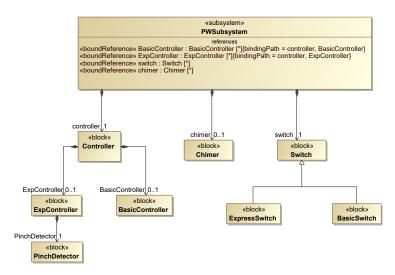
(a) SysML: Decomposition hierarchy of the power window subsystem into its individual components along with the bound references to corresponding variants.
