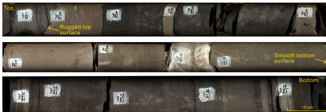
Fig. 4 Photographs of facies C showing massive sandstone with an irregular top surface and a smooth bottom surface, well Jh25, 1277.51–1280.10 m
