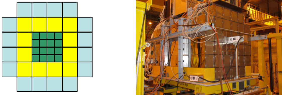
Figure 13. (Left) schematic front view of the present PSD of NA61/SHINE. (Right) Photo of the PSD placed on the beam line downstream of the NA61/SHINE detector. An additional small module (1.8 interaction length) is installed in the front of the PSD.
