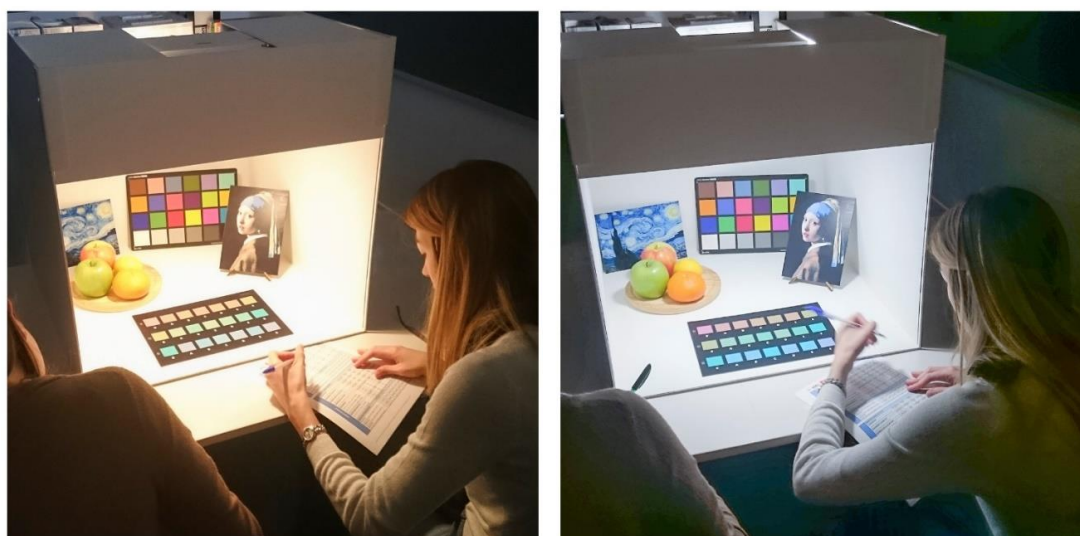
Figure 8. Analysis of color rendering of a warm and cool LED lamp in the light source testing box.
