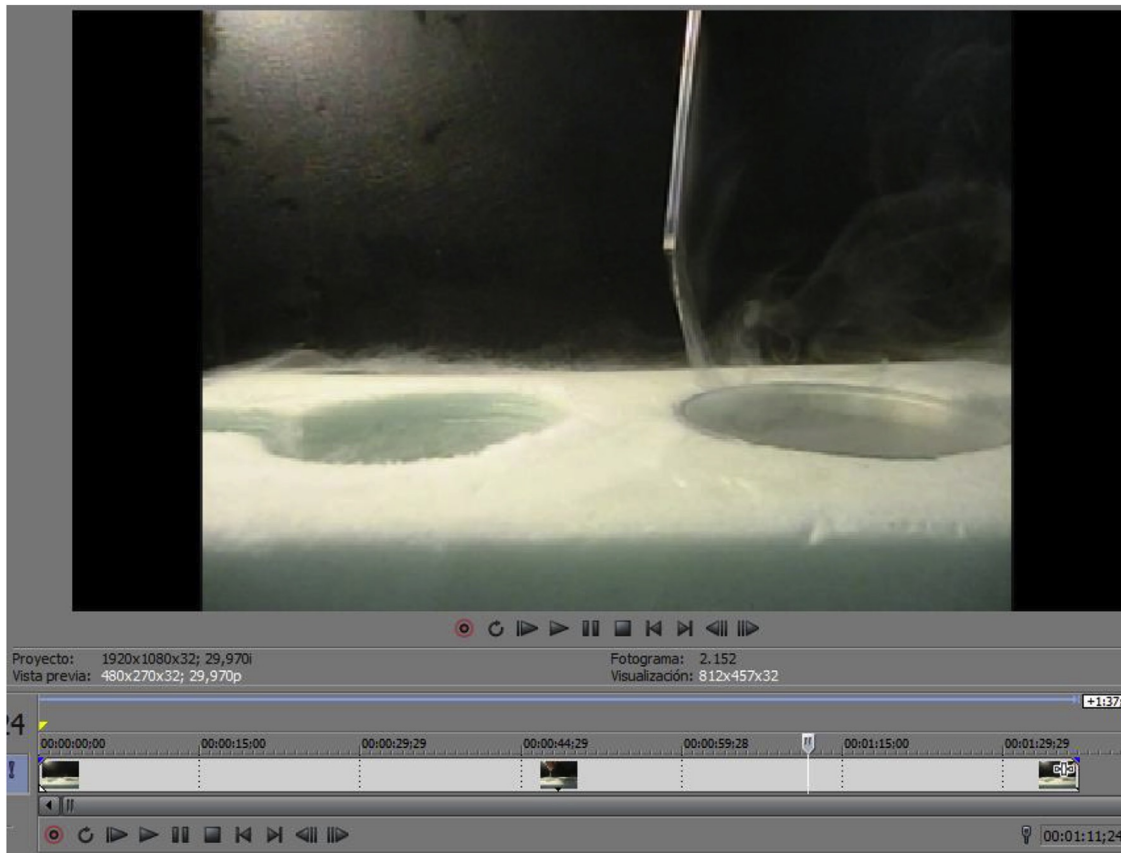
Fig. 3. Determination of the time of flight. Frame by frame visualization of the video enables (Sony Vegas software), with a temporal resolution of milliseconds, the determination of the exact lapse of time between the exit from liquid nitrogen and the entrance in the warm water bath.
