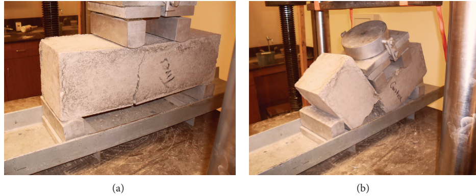
FIGURE 9: (a) Failure pattern for 7.5% TDA-1'' concrete beam. The beam did not fail into 2 halves and fracture line was not parallel to loading direction. (b) Failure pattern for Control-0% TDA concrete beam. The beam failed into 2 halves and fracture line was parallel to loading direction.
