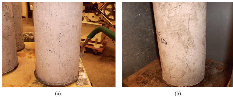
FIGURE 7: 7.5% TDA-1'' concrete failure patterns. The fracture line was generally at an angle to the loading direction.
