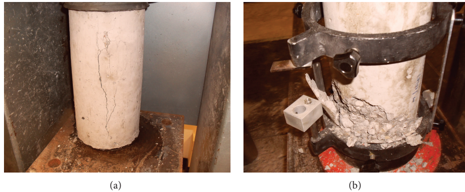
FIGURE 6: Control-0% TDA concrete failure patterns. The fracture line was generally parallel to the loading direction and failure was catastrophic.
