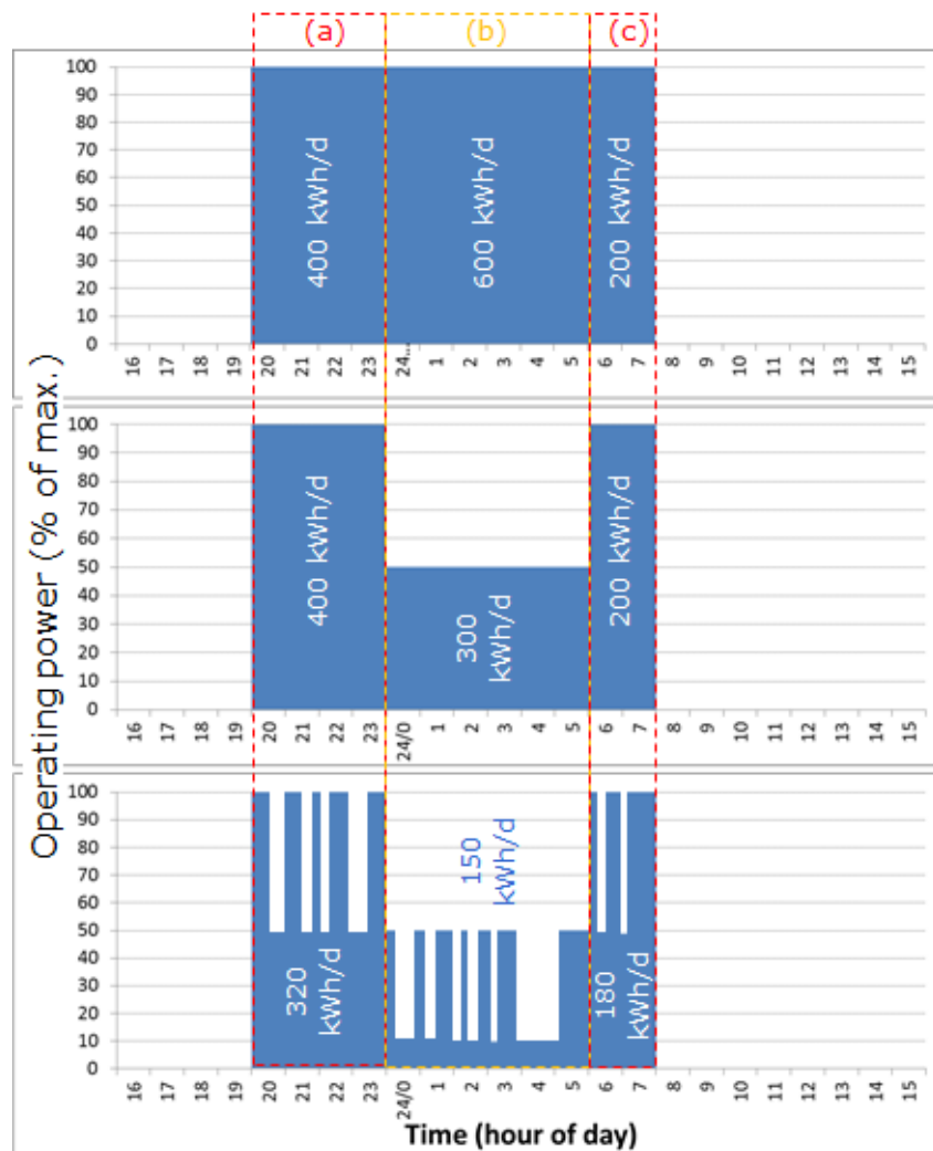
Figure 12. Examples of different operational profiles for road lighting installations during period a) evening peak hours, b) off-peak hours and c) morning peak hours (adapted from EN 13201-5). Consumption figures included refer to a 100kW installation
