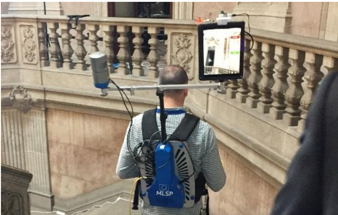
Figure 2: Using MLSP for the evaluation of a localization device: the laser scanner acquiring the ground truth data is mounted on the left. The competing device is mounted on the right.
