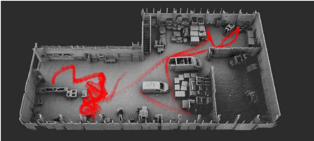
Figure 9: Results of the clean data classification. Points shaded in grey are the ones labelled as 'static', whilst red points correspond to 'moving' objects. The trails created by persons walking around during the acquisition were completely detected and, thus, removed in the final point-cloud.
