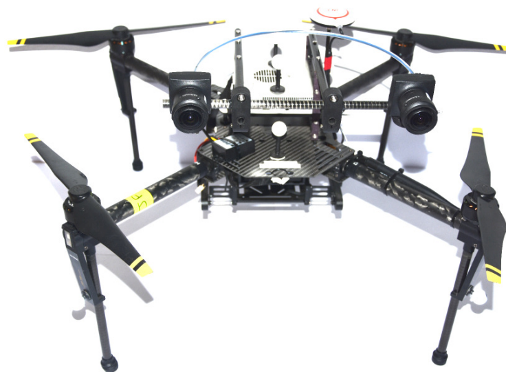
FIGURE 3.7: Housed stereo camera using UI- 1220-LE-C-HQ with Tamron lens setup fixed on the DJI-Matrice 100 UAV
