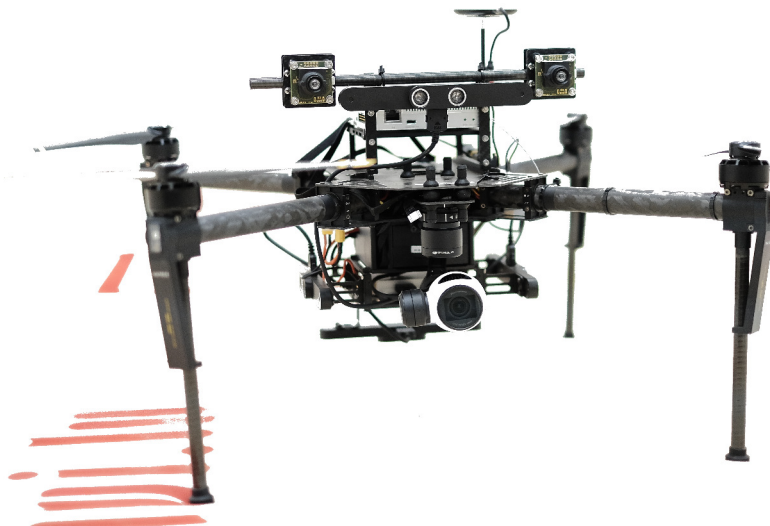
FIGURE 3.5: Board level stereo camera setup using UI-1221-LE-C-HQ fixed on the DJI-Matrice 100 UAV
