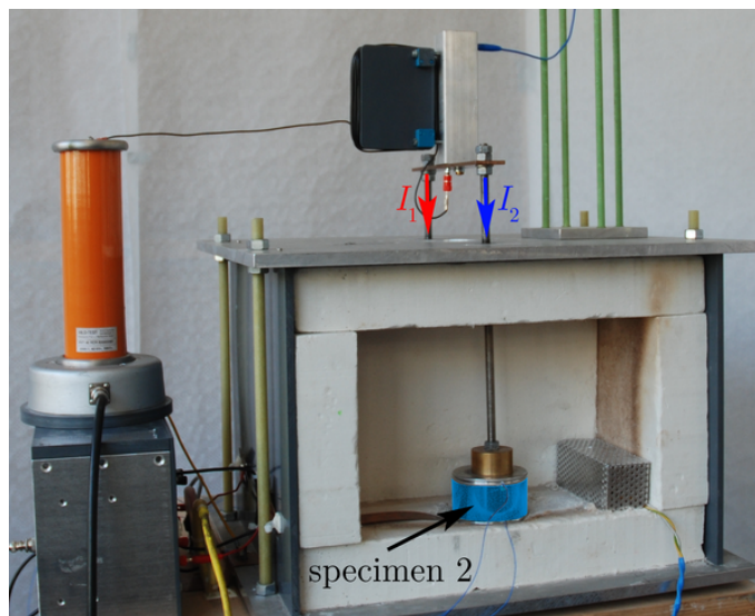
Figure 5.13: One side of the symmetrical specimen fixture for the current sharing measurement that is used for investigations of the temperature dependence within the breakdown region of the V-I characteristic.
