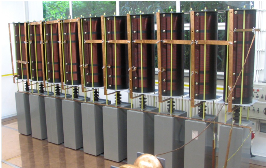
Figure A.3: The long-duration current impulse generator during the setting up with ten stages.
