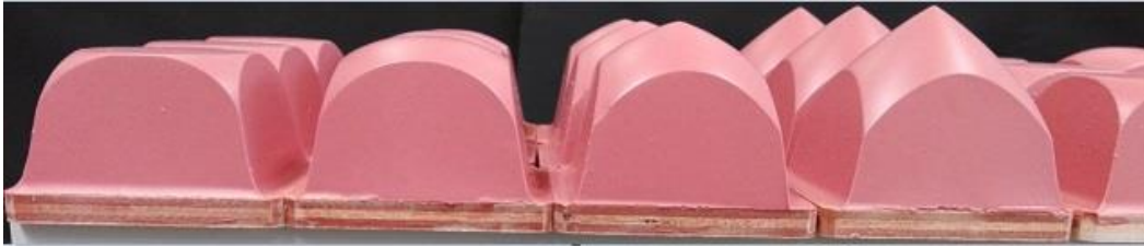
Figure 5-9: The produced silicone rubber pads. The four designed pads are produced with four different hardnesses of 3, 6, 12 and 18 Shore A. In each case three times the same pads are molded. Totally, 48 pads are produced.
