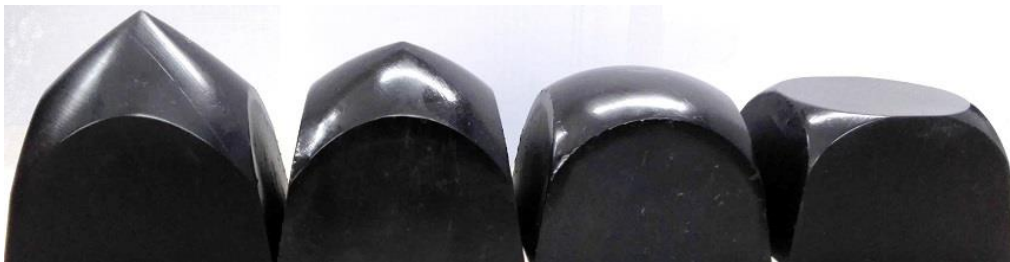
Figure 5-8: The 3D printed positive forms. They are printed after designing and drawing the desired pads.
