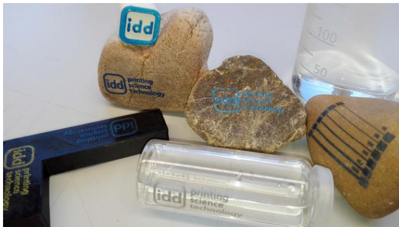
Figure 2-4: The samples with different mechanical features printed on by the use of indirect gravure printing. The substrates materials are fragile glasses with smooth surfaces, hard stones with very rough surfaces and 3D printed objects made of PLA. The printed elements are letters, logos, numbers, high accurate beakers marked lines and fine lines with different thicknesses.
