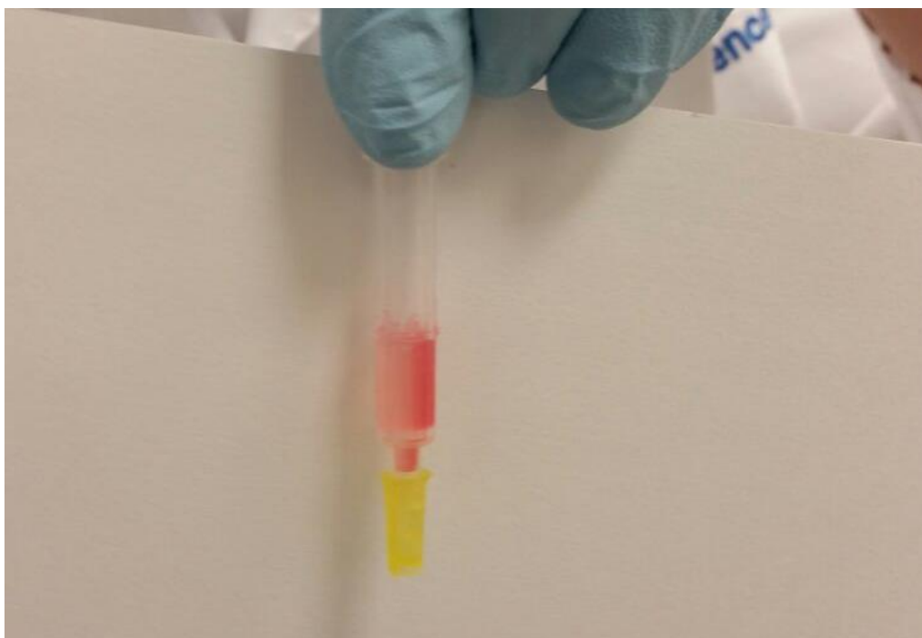
Figure 26: Irradiated Affi-gel 10 resin with mixed in marker molecule “compound 3” The column was irradiated for 60 s with UV light ( \lambda=365 nm, 0.6 A, 15 V; condition 1, Table 22) from the right side, leading to a colour gradient within the column. The “compound 3” molecules on the right side of the column have been switched in a higher percentage than the ones on the left side of the column.
