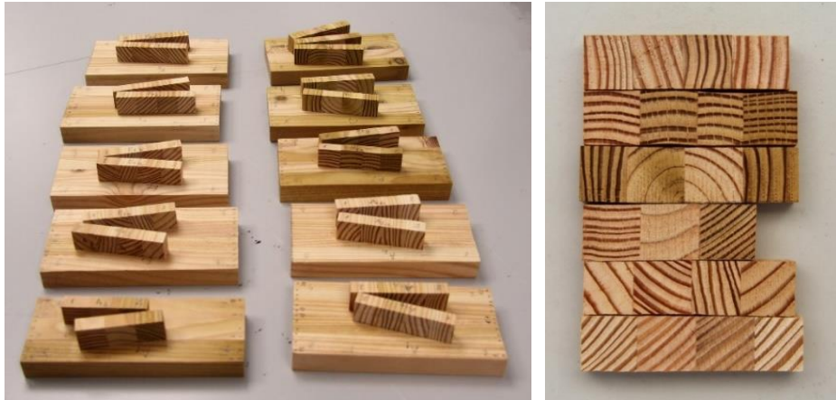
Figure 1a: Laminated samples after cutting and planing to the required thickness. Small matching samples for moisture uptake study were cut from the ends of the longer weathering samples. 1b: End grain of a selection of moisture content samples, showing matched and non-matched grain orientation within the laminate
