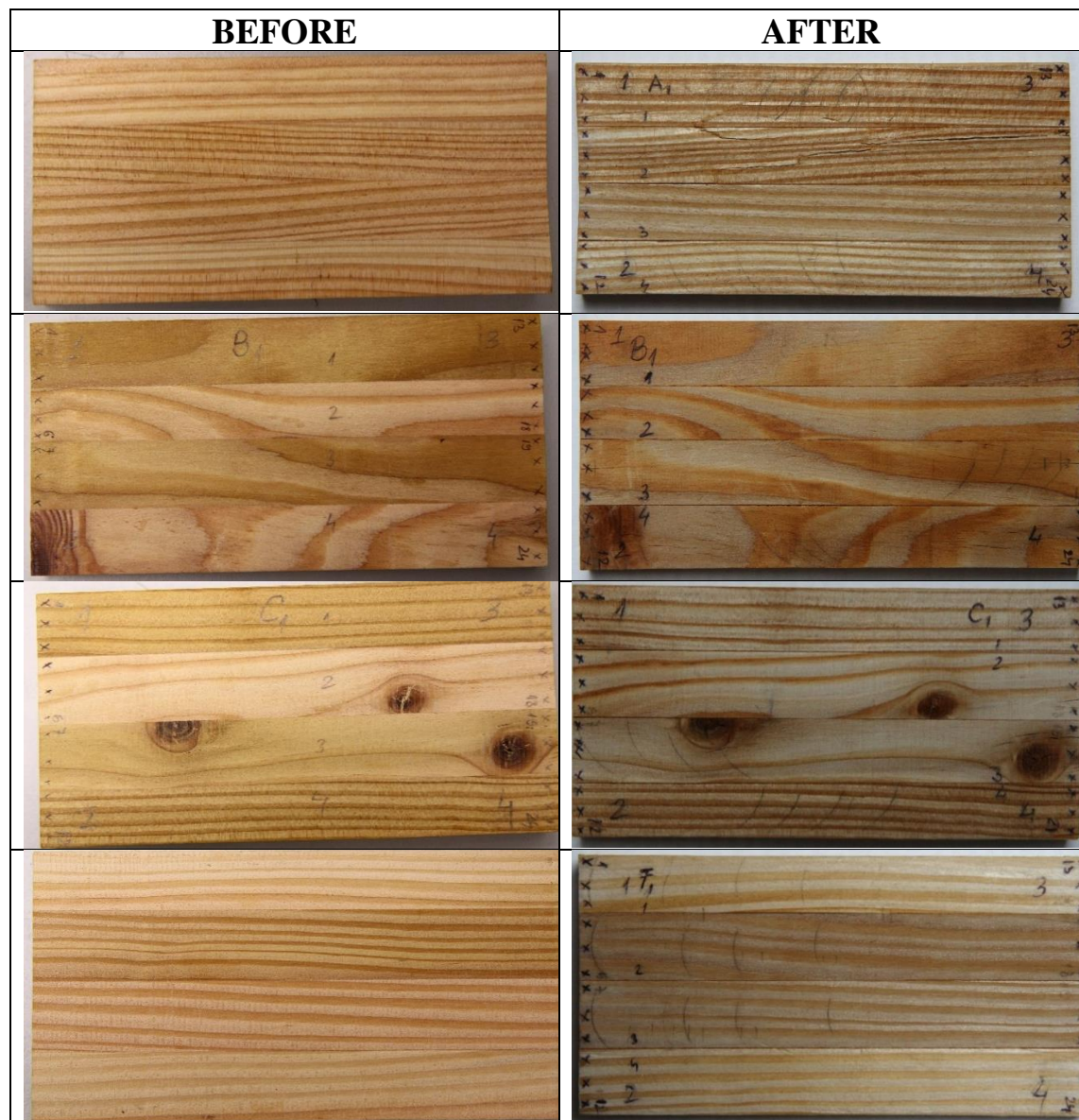
Figure 3: Photographs of samples A1b, B1b, C1b and F1b before and after QUV weathering exposure
