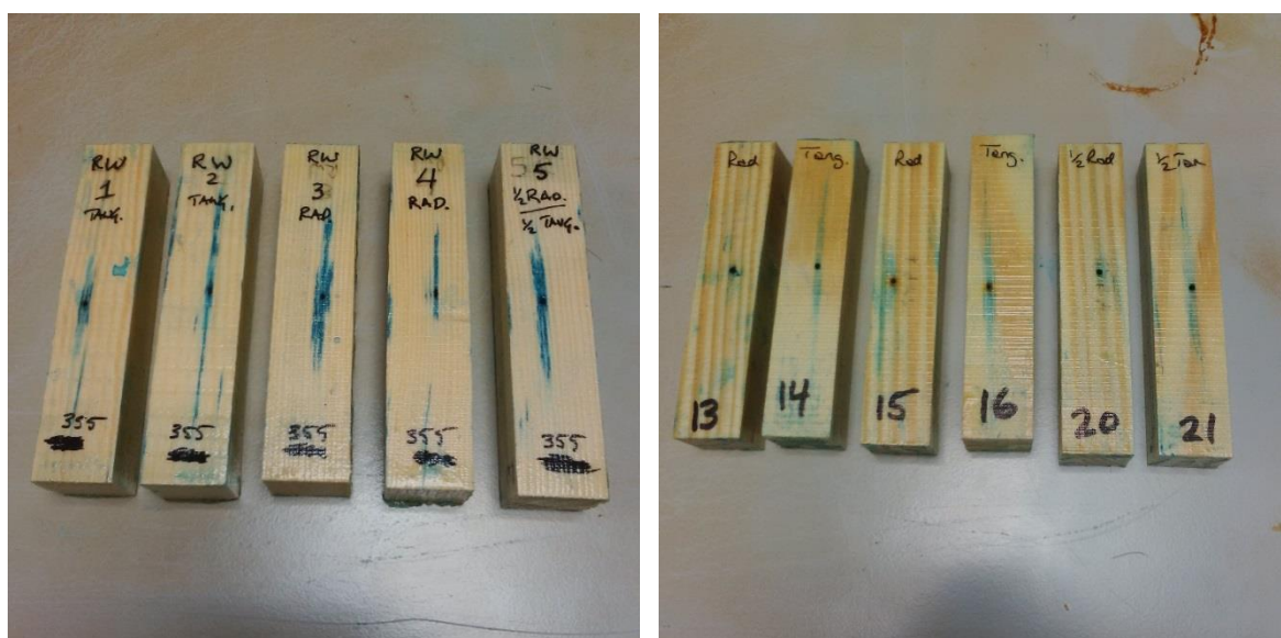
Figure 1. Samples of (a) European redwood and (b) Southern yellow pine, incised with UV laser (355nm) prior to dissection, showing extended longitudinal flow.
