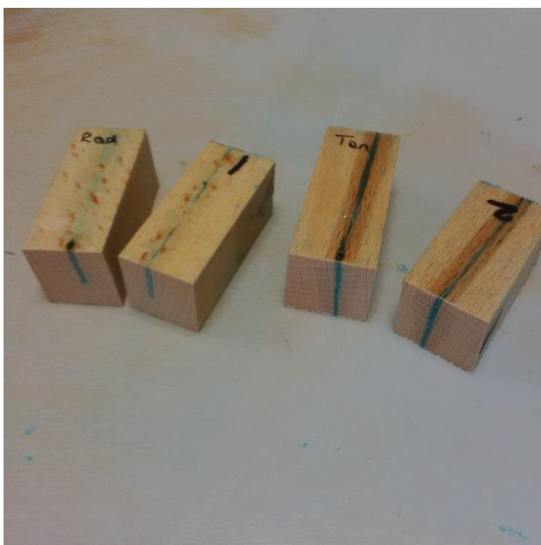
Figure 5. Samples of beech incised into the radial face (left) and tangential face (right), revealing longitudinal flow through the full length of the sample, but minimal lateral flow.
