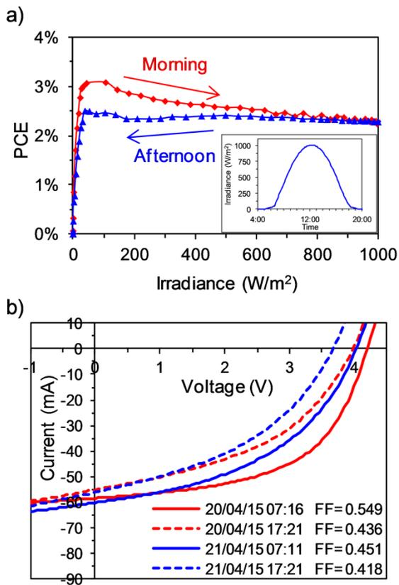
**Figure 6:** a) PCE plotted against irradiance on a sunny day (inset graph shows irradiance vs. time), highlighting the different pattern in the morning and afternoon; b) Comparison of morning (solid) and afternoon (dashed) IV curves on 2 consecutive sunny days [current linearly adjusted to  $1000 \text{ W/m}^2$ ].
