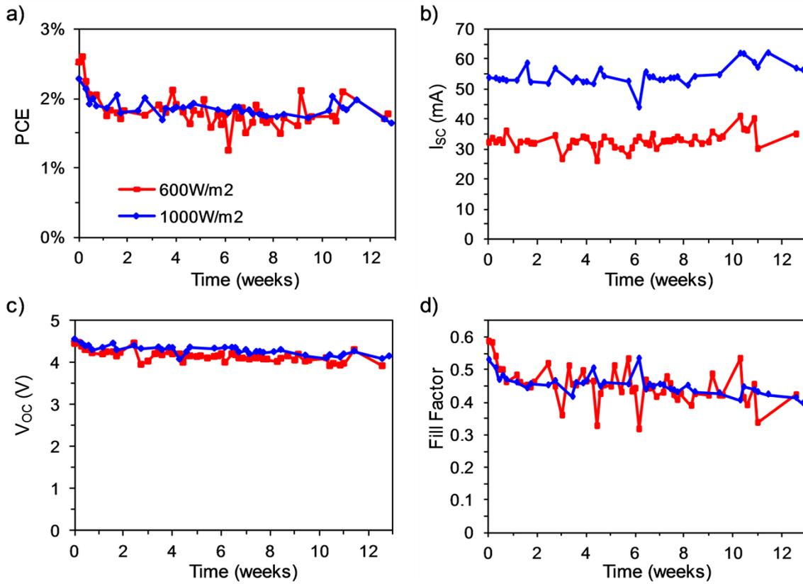
**Figure 5: Degradation of OPV modules with silver nanowire front electrodes: a) PCE; b)  $I_{sc}$ ; c)  $V_{oc}$ ; and d) FF. Measurements were selected at two different irradiances ( $600 \pm 15 \text{ W/m}^2$  and  $1000 \pm 15 \text{ W/m}^2$ ) and daily averages are plotted.**
