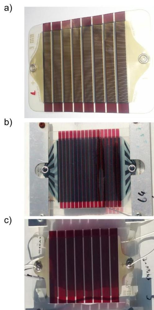
**Figure 2: DTU freeOPV modules: a) OPV(AgGrid), first generation freeOPV modules with silver grid electrodes at front and rear; b) OPV(Carbon), freeOPV module with graphite busbars; and c) OPV(AgNW), freeOPV module with silver nanowire front electrode.**
