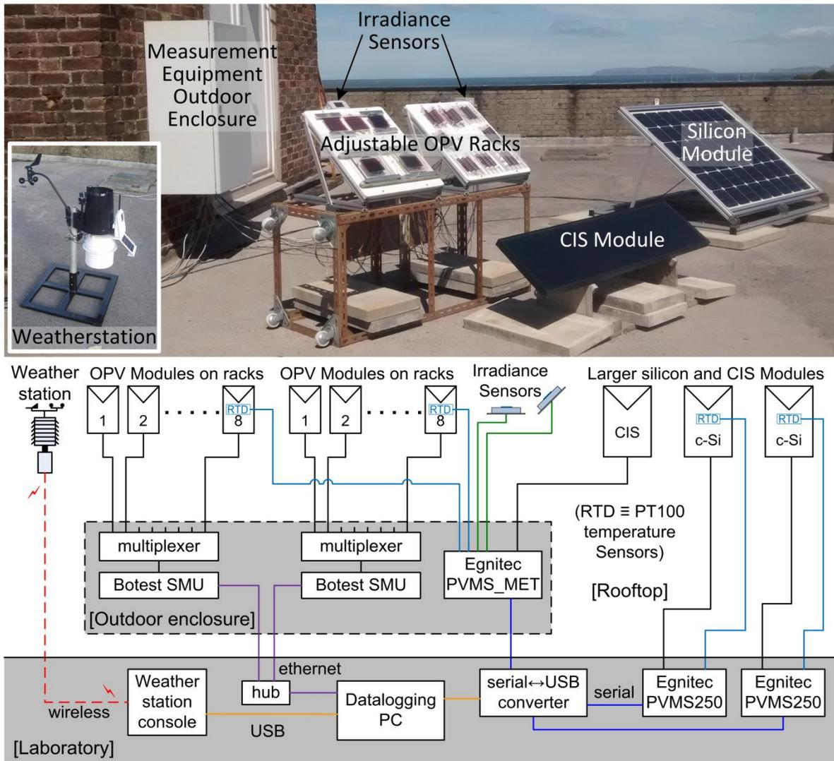
**Figure 1: Photograph (top) and system schematic (bottom) of the outdoor monitoring system on the roof of the School of Electronic Engineering at Dean Street, Bangor (inset in photograph shows the wireless weather station).**
