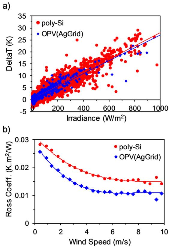
**Figure 4: a) Effect of irradiance on module temperature rise above ambient ( $T_{\text{DELTA}}$ ) plotted against irradiance with linear trend lines. The slope of each line is the Ross coefficient. b) Effect of wind speed on Ross coefficient.**
