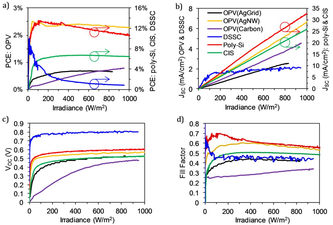
**Figure 3: Comparison of performance parameters for poly-Si, CIS, DSSC and three different OPV modules: a) PCE; b) J<sub>sc</sub> (per cell); c) V<sub>oc</sub> (per cell); and d) FF.**
