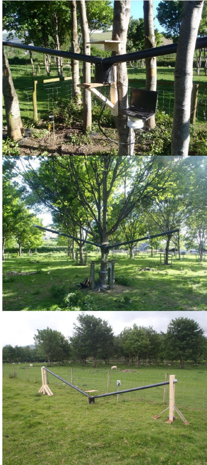
Figure 3: Throughfall and control gauges: clumped treatment (top) even spaced treatment (middle) and control gauge.
