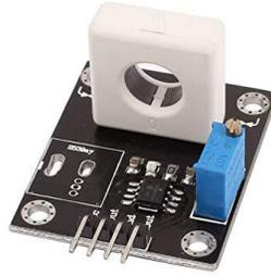
*Figura 2. 10 Sensor WCS1800 -Hall Effect Base Linear Current Sensor.*
