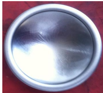
Figure 58: Bottom after stamping and application of rubber (Outer area)
