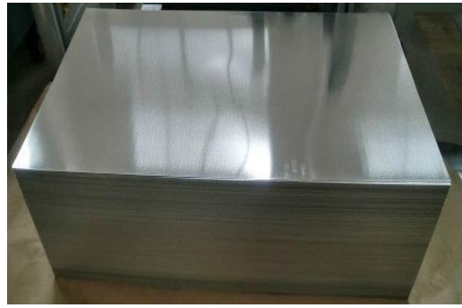
Figure 49: Rectangular tinplate after the cutting process
