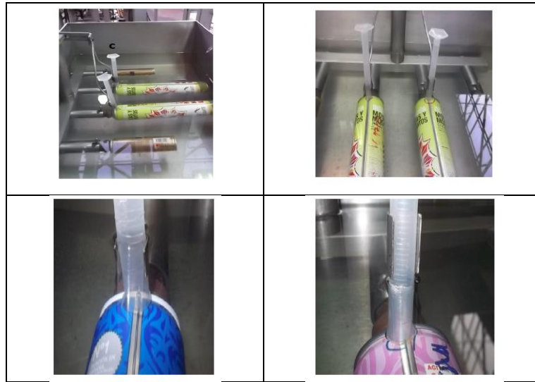
Figure 26: Examples of manual waterbath leak testing (Teixeira 2013)
