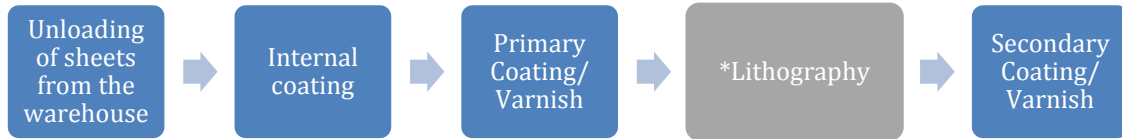
Figure 50: Breakdown Process for Coating/Varnishing (* Lithography is not a part of the varnishing process)
