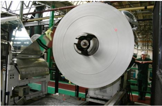
Figure 48: Coil cutting process
