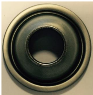
Figure 55: Top after stamping and application of rubber (Outer area)
