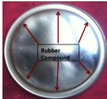
Figure 59: Bottom after stamping and application of rubber (Inner area)
