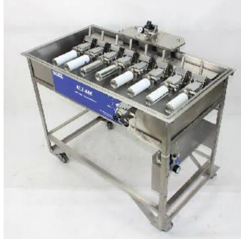
Figure 25: Illustration of manual waterbath method (8 heads – Colep has 6 heads machines)
