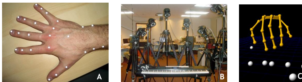
Figure 2.19 - Example of a Vicon passive motion capture system. The figure illustrates a study carried out by MDW (University of Music and Performing Arts Vienna), where the passive markers are found in A, the configuration of infrared cameras in B and the respective output in C [85].
