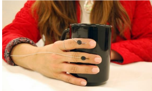
Figure 2.16 - Magnetic tracking sensors. In this figure can be seen the Polhemus sensors [84].
