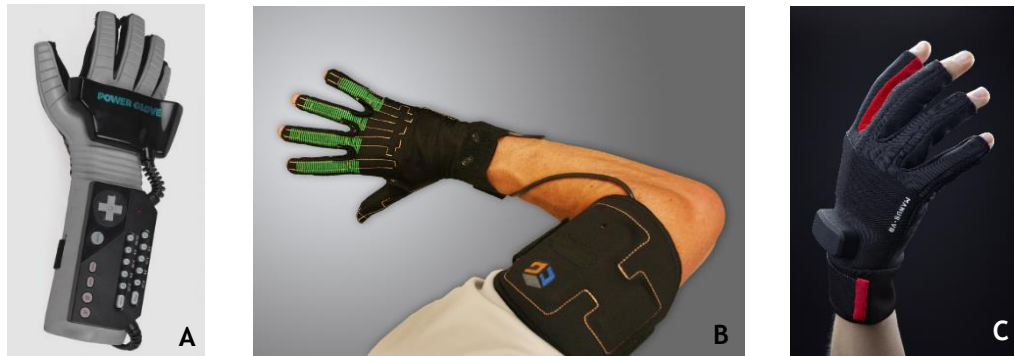
Figure 2.12 - Datagloves based on flexible flex sensors (I). In this figure are illustrated the Power Glove in A, the CyberGlove III in B and Manus VR glove in C [64, 66, 67].
