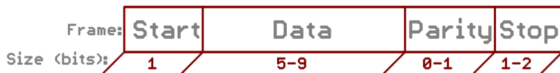
Figure 3.12- Serial packet architecture [143].
