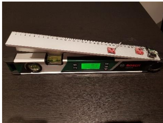
Figure 3.16 - IMUs placed in the Bosch sensor (model PAM 220).
