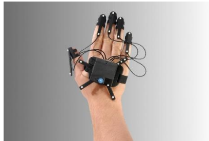
Figure 2.18 - ART active finger tracking device. In this figure is illustrated the 5 fingers version [82].
