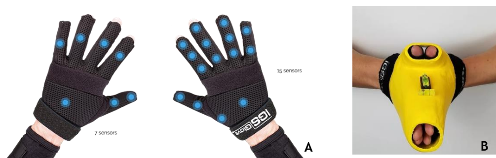
Figure 2.14 - Datagloves based on inertial tracking. In this figure are illustrated the IGS Cobra Glove from Synertial with the respective sensors location in A and Synertial's Calibration Pipeline in B [73, 74].
