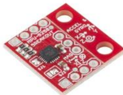
Figure 3.3 - Inertial Measurement Unit MPU-9250 [131].
