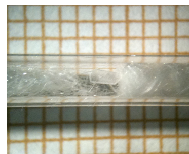
Figure 3. Crystal 2, mounted in its glass capillary. The broad upper face is (010) and the edge parallel to the bottom of the image is (102).
