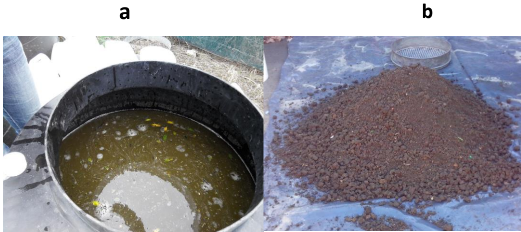
Figure 4. 2 (a) Homogenising of DSE and: (b) biosolids used in the experiment Plate 4. 2 (a) Homogenising of DSE and: (b) biosolids used in the experiment
