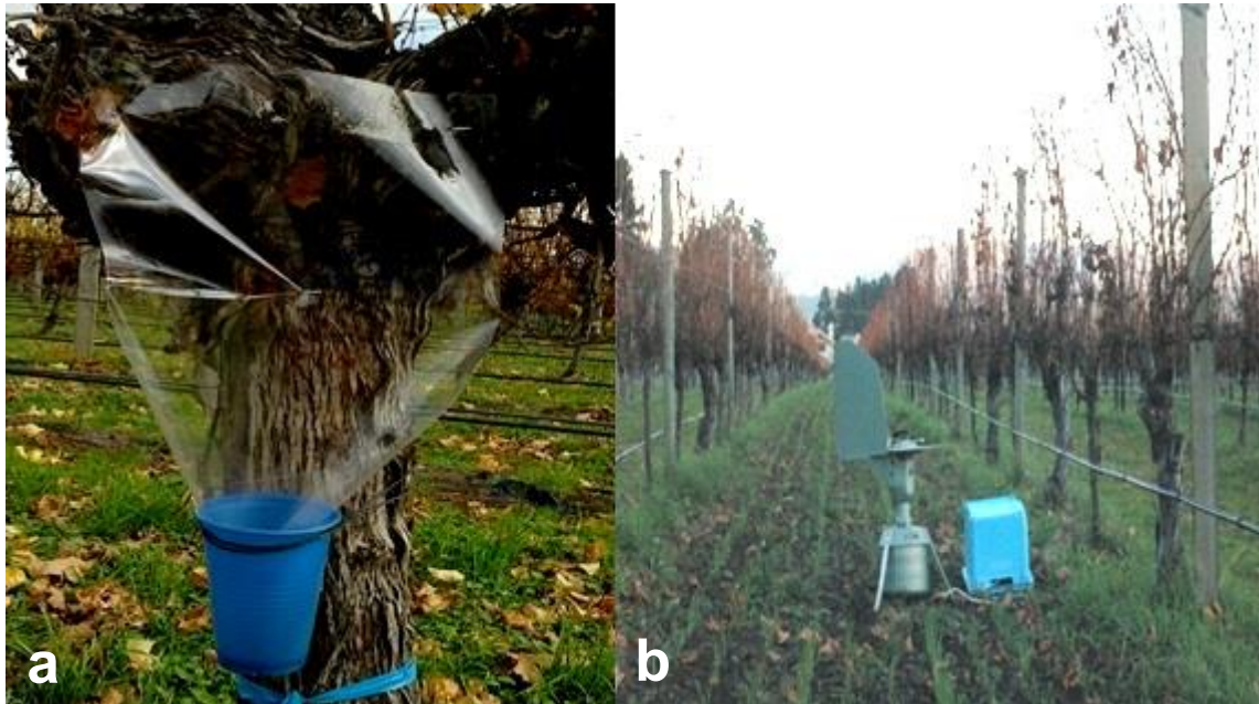
Figure 3.1 (a) Rain water spore trap, (b) Burkard spore trap placed in the vineyards to trap air-borne spores of Botryosphaeriaceae species.
