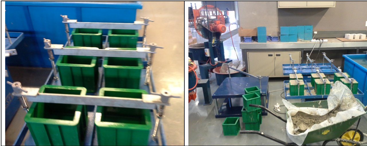
(a) (b) Figure 3.6: (a) Concrete mould clamped to the vibrating table (b) Concrete specimen on the vibrating table during vibration
