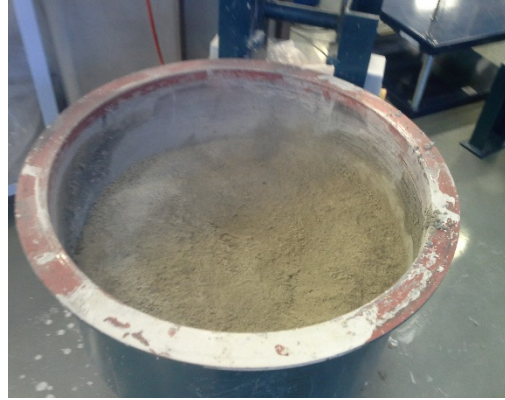
Cement constituents in a 50 L Drum
