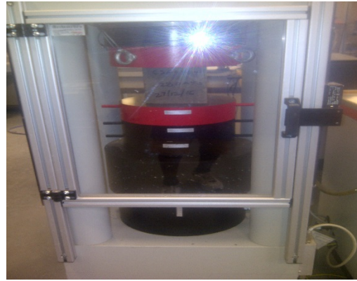
Sample under crushing at 90 days
