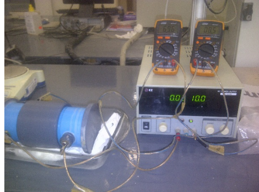
Chlorine Conductivity exp. set up
