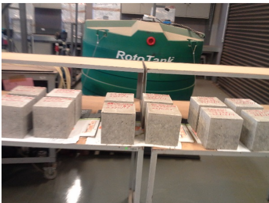
Fresh concrete ready to be transferred Into curing tan
