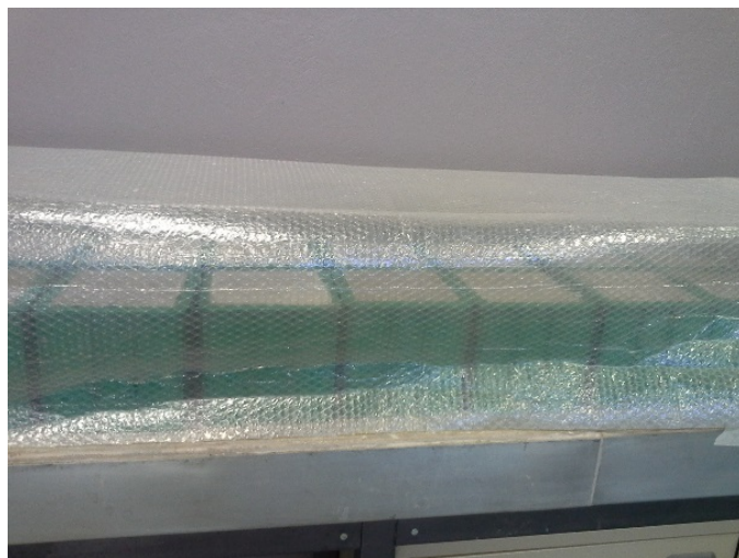
Figure 3.3b Concrete covered with polythene material
