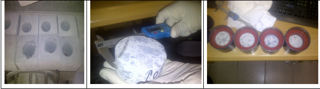
Figure 3.8: (a) (b) (c) Core drilled concrete specimens
