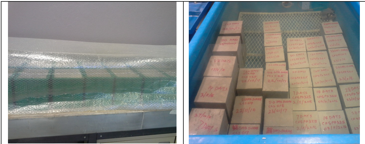
(a) (b) Figure 3.7 (a) Fresh concrete covered with impervious material (b) Concrete specimen in a temperature control-curing tank
