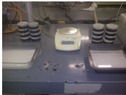
Disc specimen sealed with tape
