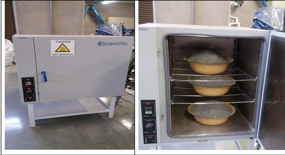
Figure 3.2: Aggregates in an oven dry process for 24 hours prior to casting
