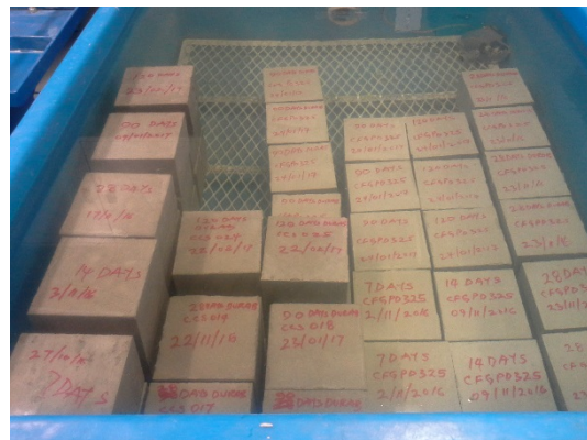
Concrete samples in a curing tank
