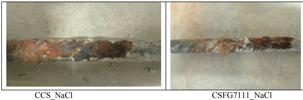
Figure 4.19: physical observations of reinforced concrete samples cured in Sodium Chloride
