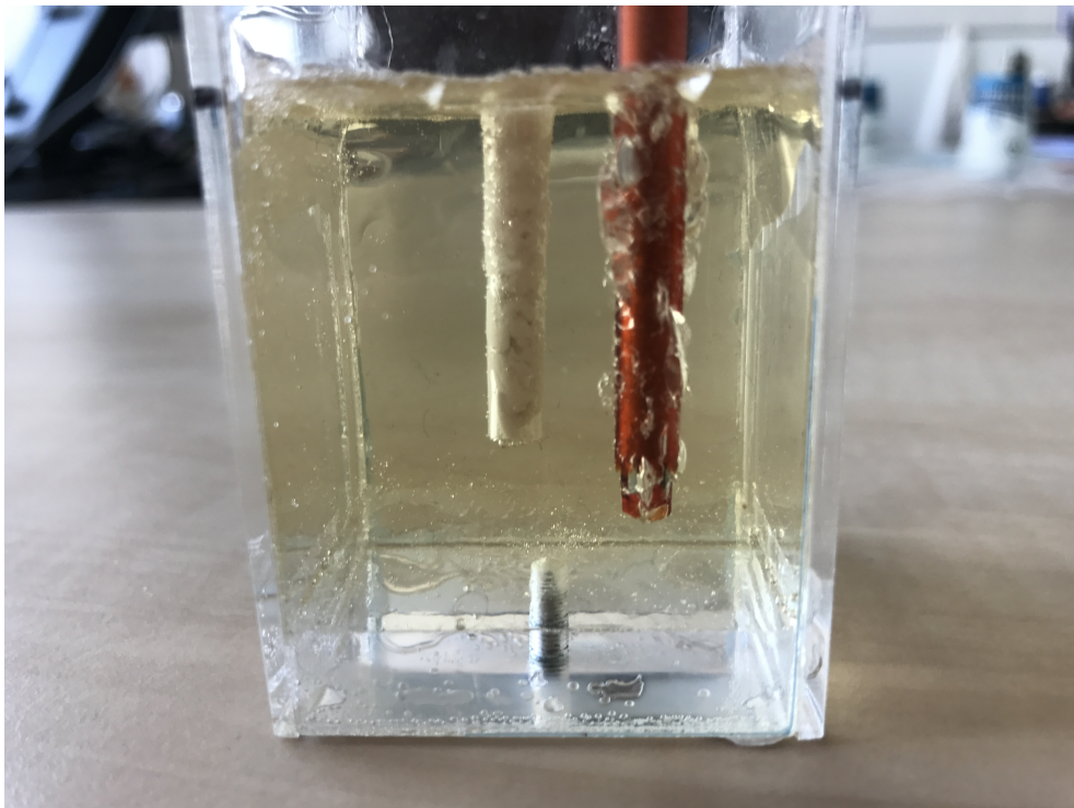
Figure 5.4: The assembled device was tried on gelatin to see if it was able to cut through soft tissue
