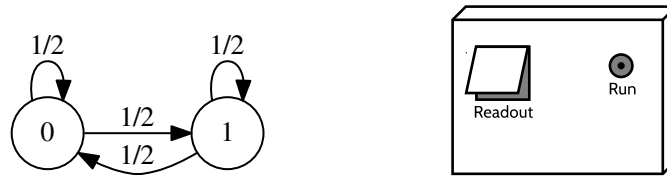
Figure 4: A simple automaton which, when run, randomly transitions to one of two possible states. In the state-transition diagram at the left, edge labels represent probabilities for the indicated transitions.
