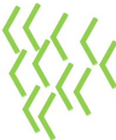
Figure 30 A cartoon of a biaxial nematic phase with orientation along both vertical and horizontal axis.
