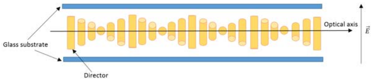
Figure 17 The ULH structure of chiral nematic liquid crystal in a homeotropic cell with the optical axis along the helical axis.
